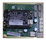
Integrated control board with micro usb (Amlogic A113D)
