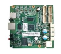
Combined control board, it's composed of IO board and BB board
