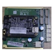
Integrated control board(A113D Control board), need to use the OTG cable (Micro usb - USB A)
